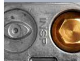
*External oil and inspection plugs put an end to dismantling the entire pump to perform a simple seal-condition check and oil change.*
