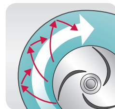
Standard impeller slams solids into the volute.
