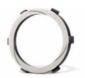
**ACTIVE SEAL™** technology from Flygt enhances sealing reliability by making the inner seal in a double seal system act as a micro pump. Laser-cut spiral grooves in the seal face of the inner seal pump liquid from the inner to the outer diameter of the seal ring, thus preventing liquid from entering the stator housing.
