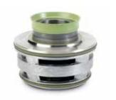
**PLUG-IN SEALS™** feature two independent mechanical seals (inner and outer) mounted in a single ready-to-install unit. No special service tools are required for installation and intelligent design protects sensitive sealing surfaces and springs from impurities. Selected variants feature our patented and leakage-preventing Active Seal technology.
